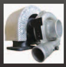
The four brackets supplied with the kits will need to be bent into shape in order to mount the shield. Fit the four brackets loosely using the dump pipe, oil/water flanges or the centre bearing bolts, so that they supply four
